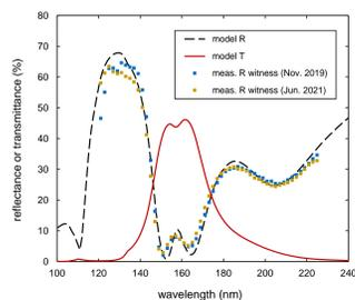
Fig. 2. The measured reflectance of witness samples to the device in Fig. 1 and the model target and predicted transmittance. Little change in witness reflectance is observed for long duration storage.
