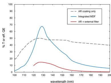
Fig. 3. The modeled performance of a directly integrated metal-dielectric filter (MDF) versus a simple AR coating, and an AR + stand-alone filter optimized for a bandpass near 130 nm.
