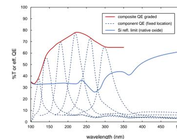
Fig. 7. Metal-dielectric structures that incorporate graded thickness can significantly improve throughput over bare Si devices in the FUV. The modeled QE shown here is for a simple three layer filter with a single graded layer of AlF<sub>3</sub> capped with uniform layers of Al and AlF<sub>3</sub>.
