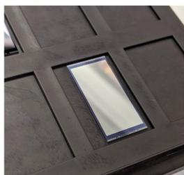
Fig. 1. A delta-doped Teledyne e2v CCD with an integrated metal dielectric bandpass filter. The filter structure combines three Al layers deposited by evaporation with four AlF<sub>3</sub> layers deposited by ALD.
