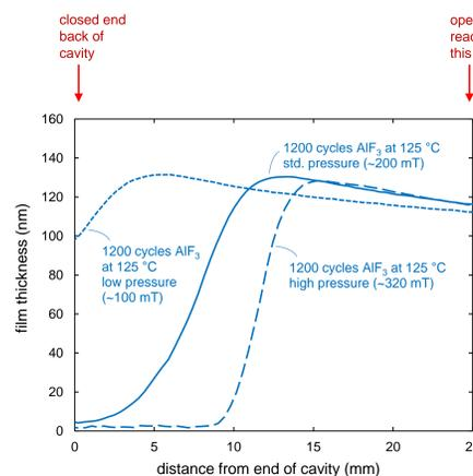
Fig. 5. Measured variation in AlF<sub>3</sub> film thickness as a function of distance into the cavity. The penetration depth can be varied by altering the height of the cavity or the working pressure of the process as shown here. Arbitrary positive slopes can be engineered by combining ALD cycles at different pressures.
