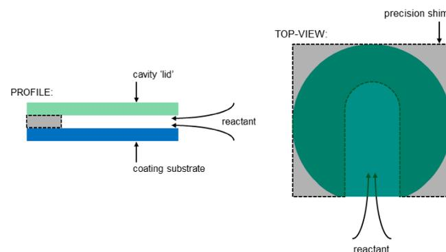
Fig. 4. Deposition into a shallow cavity limits the amount of reactant that can penetrate before the next ALD half cycle begins.
