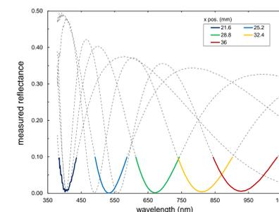
Fig. 6. (upper left) The modeled transmission (red curve) of the three layer AR coating on Si shown in the inset. (upper right) The measured spatial variation in Al<sub>2</sub>O<sub>3</sub> thickness for this three layer coating deposited by the ALD cavity method on a Si wafer. (bottom) The measured spectral reflectance of the three-layer stack at various points along the graded direction.
