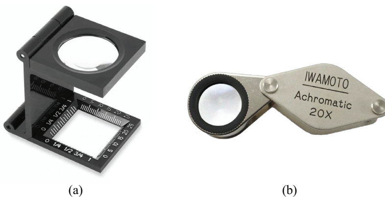
Figure 1.76 Optical magnifiers. (a) A Carson LinenTest™ 5\times loupe magnifier with a base on the focal plane of the lens. Image reprinted from https://carson.com/ with permission from Carson. (b) An Iwamoto wide-field 20\times magnifier with three lenses in place to correct chromatic aberration. Image reprinted from https://www.ascscientific.com/ with permission from ASC Scientific.
