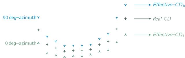
**Fig. 17** A sketch schematically illustrating the main finding: in a scatterometric CD measurement, the real CD value is only to be found between two effective-CDs measured at two perpendicular polarizations. To create this sketch, we use data similar to data you can find in Fig. 16.
