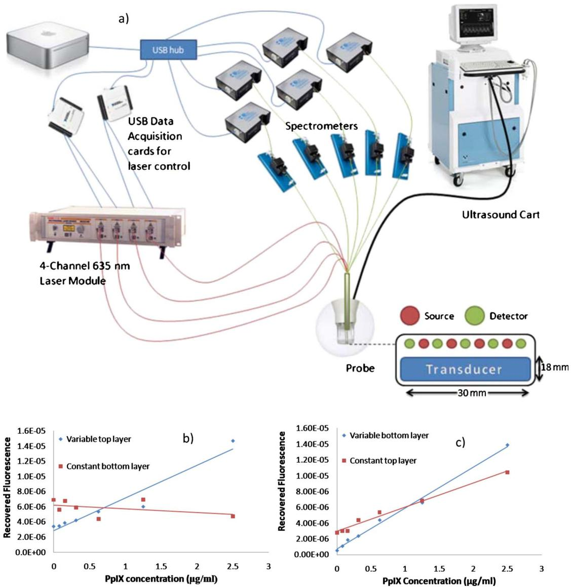
**Fig. 1** The system schematic is illustrated in (a) showing components and probe geometry, with data acquisition from five compact spectrometers. The recovered fluorescence values for the layers (b) with the top concentration varied and the bottom fixed at  $0.625 \mu\text{g/ml}$ . In (c), the top layer was held constant and the bottom layer varied.
