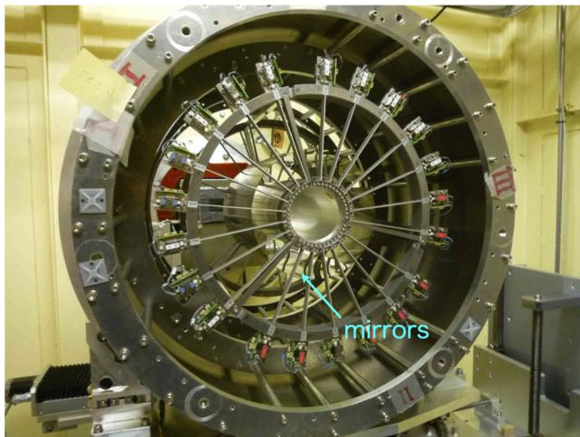
**Fig. 9** The setup of the 200-mm diameter mirrors in the housing, viewed from the bottom side at BL20B2. The collimated x-ray beam enters the mirrors from the back side in this picture.
