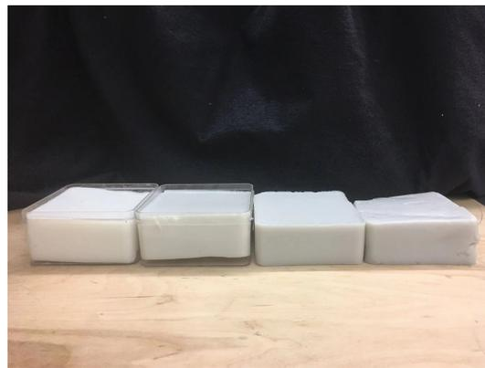
**Fig. 4** Four high contrast solid phantoms for mimicking the chest wall with the size of 10 cm by 10 cm by 4 cm. Their absorption coefficients range from 0.095 to 0.18, and their reduced scattering coefficients range from 5.6 to 7.1 cm<sup>-1</sup>.
