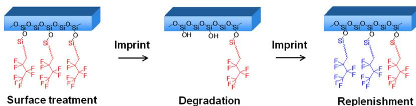
Fig. 5 Replenishing the release layer.
