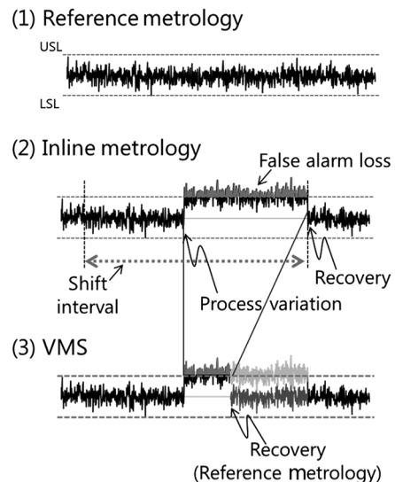
**Fig. 8** Cost model for false alarm case.
