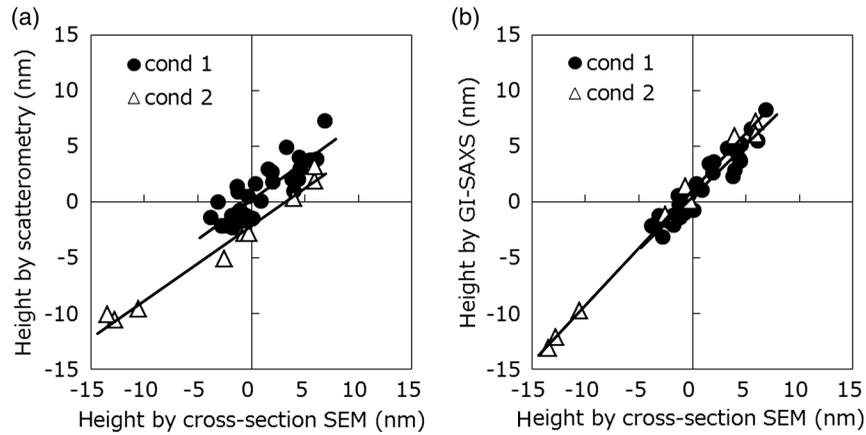
**Fig. 6** Measurement robustness of scatterometry and GI-SAXS: (a) scatterometry result and (b) GI-SAXS result.
