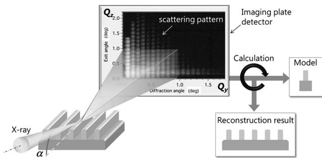
Fig. 4 Schematic diagram of GI-SAXS.
