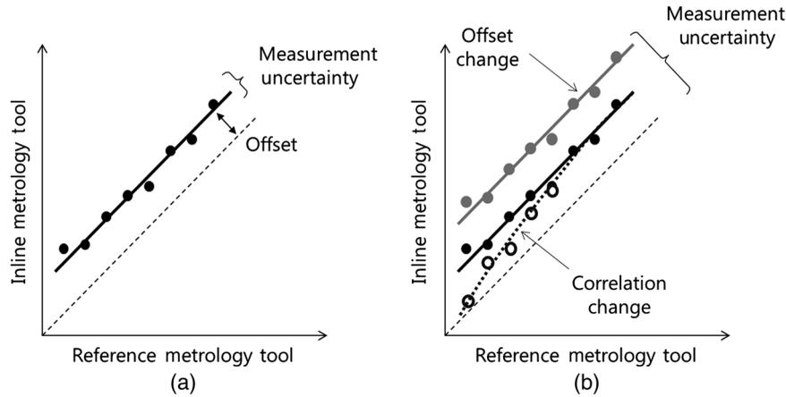
**Fig. 1** Measurement uncertainty (MU) for ideal and actual pattern shapes: (a) ideal pattern shape without process variation and (b) actual pattern shape with process variation.
