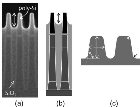
Fig. 5 Structural models for scatterometry and GI-SAXS: (a) cross-sectional SEM image, (b) scatterometry model, and (c) GI-SAXS model.
