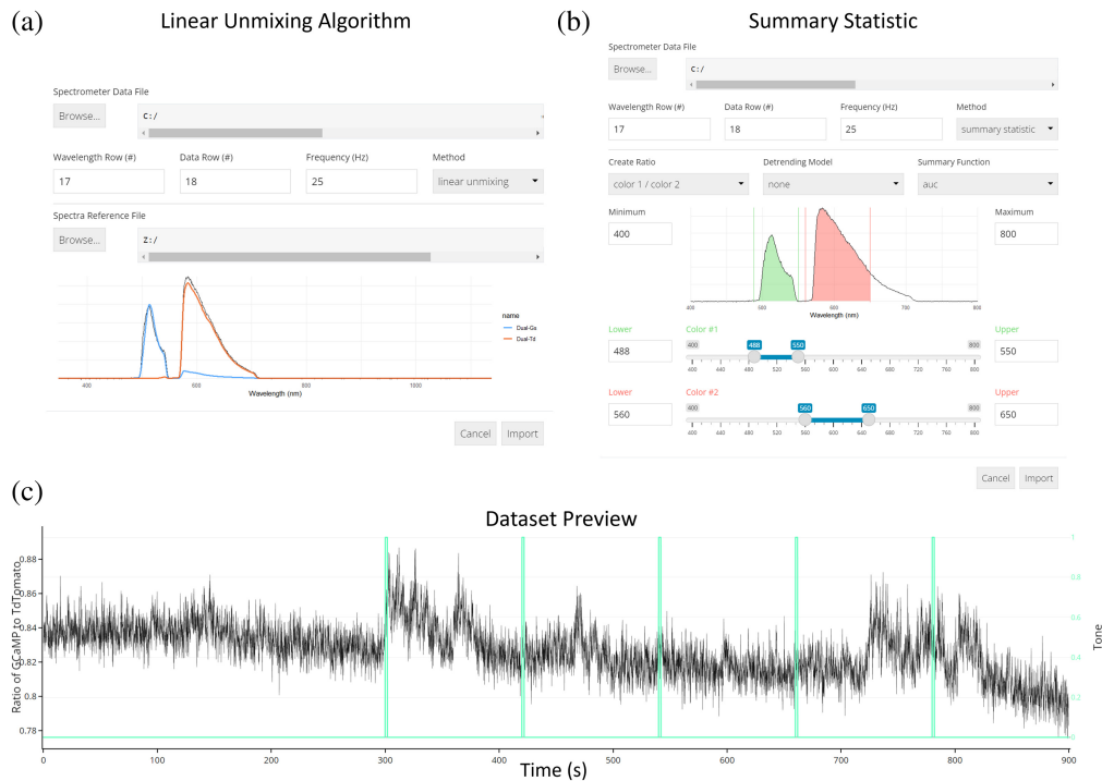
Fig. 2 Import options for data collected using spectrally resolved photometry systems. (a) The linear unmixing algorithm showing a GCaMP and tdTomato fluorescence peak as well as a reference spectrum. (b) Importing data using the summary statistic option with calculating the area under the curve. (c) Dataset preview of a 900 s photometry recording session aligned with TTL pulses of five tone presentations.
