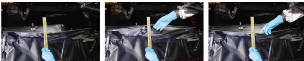
**Fig. 19** Frill blanket inspection measured the slack when a force was applied normal to the edge of the seam between adjacent blankets. This inspection method confirmed that many locations did not have the designed slack.
