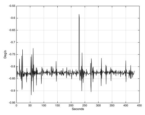
Fig. 2 Counterclockwise test starting from 90 deg (slit east) running 360 deg, showing velocity variations related to mechanical problems that may indicate incipient failure.
