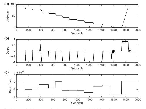
Fig. 1 Counterclockwise test starting from 90 deg (slit east). (a) Azimuth integrated from velocity (b) using computed bias offsets (c).
