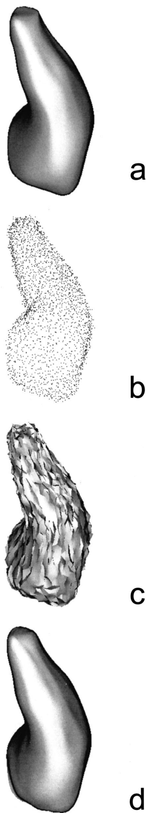
Fig. 6 Simulations with the test surface. (a) The original test surface (synthesized surface) with a shape and dimensions similar to these of a real ear canal impression. (b) The noisy range data obtained by adding a Gaussian noise of 0.177 mm (rms value) to the coordinates of the vertices of the original test surface in (a). (c) A solid representation of the noisy surface. (d) The reconstructed surface obtained with the proposed algorithm by processing the noisy range data in (b).
