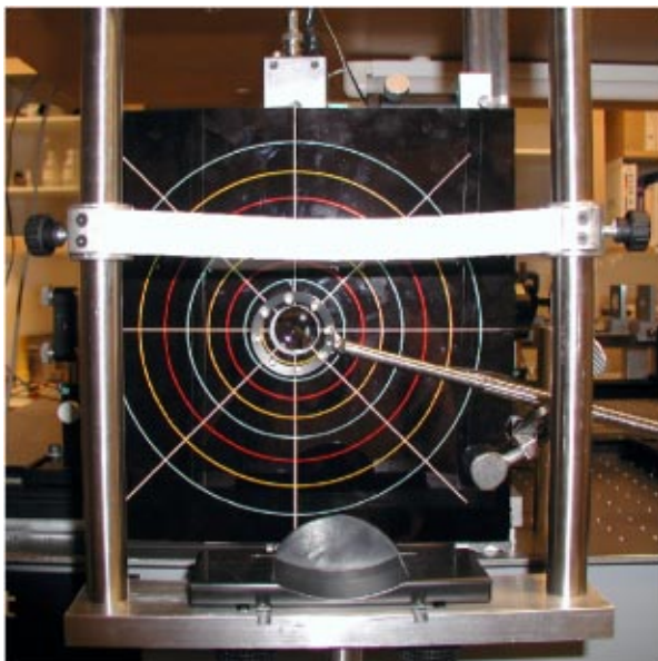
Fig. 3 The fixation target with ring patterns seen through the headrest.
