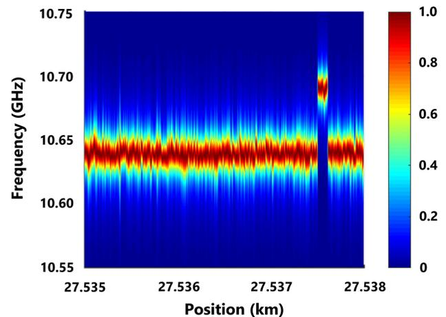
**Fig. 1** Distribution of Brillouin gain spectra measured by the long-range chaotic BOCDA system. The figure demonstrates the successful detection of a 10-cm-long strained section located near the distal end of a 27.54-km-long sensing fiber. Remarkably, the system achieves an exceptional spatial resolution of 2.69 cm, resulting in an impressive number of effective resolving points reaching 1,020,000. Figure adapted from Ref. 12.
