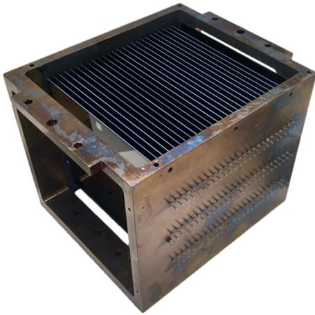
**Fig. 3** The WRXR flight grating module. 26 gratings were individually aligned into the module, each separated by  $\sim 3.8$  mm. A small optical grating square is visible on the first grating in the array; optical gratings were used in the alignment process to constrain yaw.
