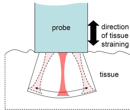
**Fig. 5** Schematically shown OCT-probe head in which scanning in the lateral direction is ensured via optical-beam tilting. The transparent output window of the forward-looking scan serves as a rigid piston to produce the tissue straining.
