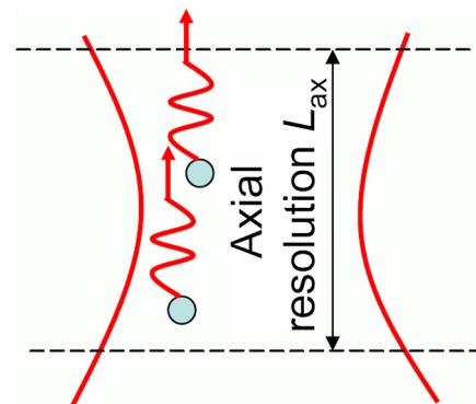
**Fig. 7** Schematically shown subresolution scatterers located within the resolution volume of an OCT system. The peculiar speckle structure is due to interference of the optical waves scattered by such subresolution scatterers with random coordinates localized within the resolution volume.
