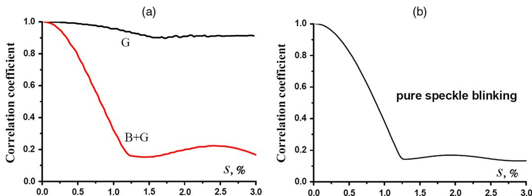
**Fig. 8** Simulation results illustrating speckle-level decorrelation. (a) Strain dependences of the correlation coefficient for the case of purely geometrical distortion of the speckle spots without speckle blinking (curve G) and for the joint effect of speckle blinking and geometrical distortions (curve B+G). (b) A similar curve obtained by retaining only speckle blinking and excluding geometrical distortions in the simulation.
