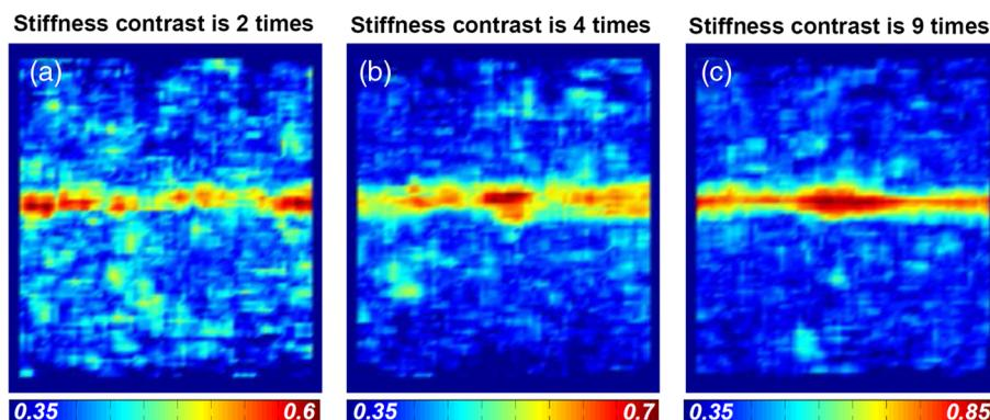
**Fig. 4** Simulated examples of correlation stability (CS) mapping of the stiffness-contrast layer. The contrast in the shear modulus between the layer and surrounding material is  $b = 2, 4$ , and 9. The average correlation maxima within the stiffer layer are  $\langle C_L^m \rangle = 0.5, 0.6$ , and 0.75 for panels (a), (b), and (c), respectively. The average value of the correlation maxima for the surrounding tissue is  $\langle C_{bg}^m \rangle \approx 0.3$  to 0.35 in all cases.
