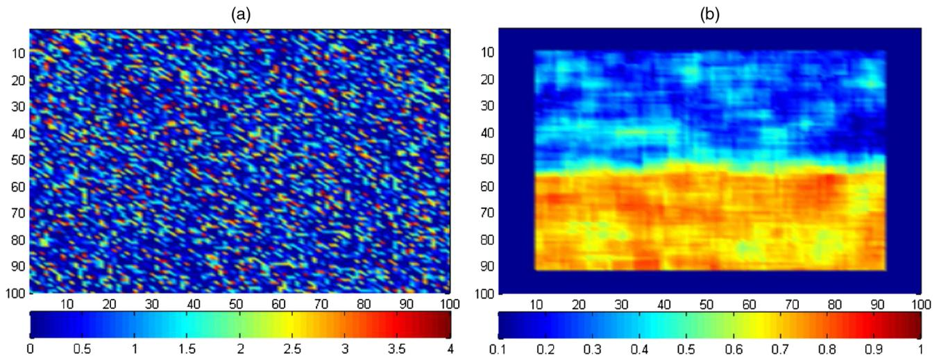
**Fig. 9** (a) Numerically simulated speckle-pattern exhibiting strain-induced blinking (Video 1) for a two-layer sample with the stiffness contrast  $b = 2$  and (b) the corresponding elastographic CS map obtained for the average strain  $s = 1\%$ . Video 2 shows the gradual strain-induced decorrelation. (Video 1: MPEG, 6.5 MB [URL: <http://dx.doi.org/10.1117/1.JBO.19.2.021107.1>] and Video 2: MPEG, 6.5 MB [URL: <http://dx.doi.org/10.1117/1.JBO.19.2.021107.2>]).
