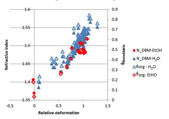
**Fig. 4** Refractive index  $(n_{\rm DBM})$  and  $\phi_{\rm org}$  versus relative deformation: an example of the  $n_{\rm DBM}$  and  $\phi_{\rm org}$  plotted against the relative deformations. Relative deformation was calculated using Eq. (3).
