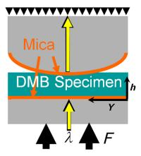
**Fig. 1** Compressive loading (F) of demineralized bone within surface force apparatus: collimated white light ( $\lambda$ ) is passed through specimens during compression. The resulting light was directed into a spectrometer and analyzed with multiple beam interferometry to determine the refractive index ( $n_{\rm DBM}$ ) and thickness (h) of the specimen. "Y" shows the direction over which the interference patterns are visualized (Fig. 2).
