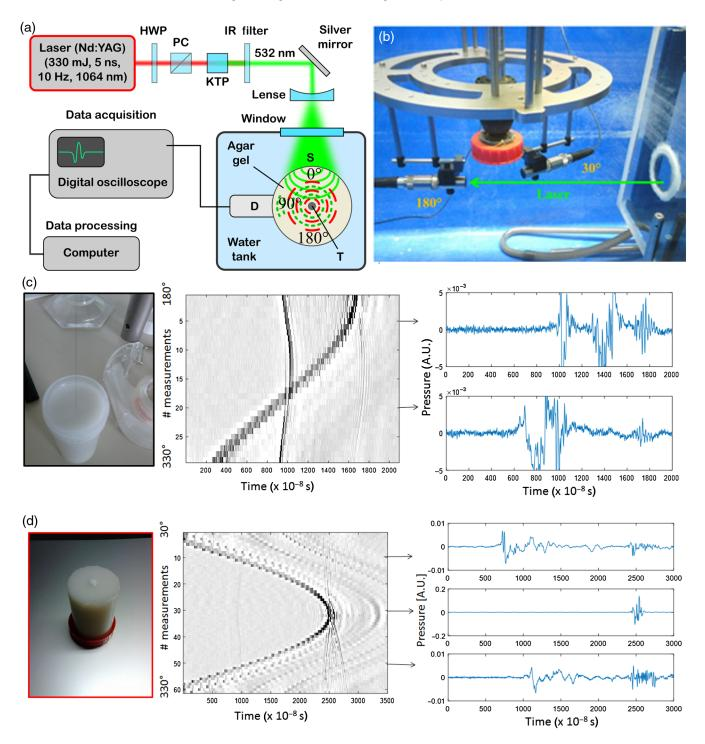
**Fig. 3** (a) Schema of the experimental setup; (b) photograph of the tranducers and phantom holder; (c) phantom containing hair inclusion: photograph, sinogram of the 32 measurements from 180 deg (transmission) to 330 deg, and two extracted crossplots; (d) phantom containing a purely acoustically contrasted inclusion, sinogram of the 64 measurements from 30 deg (reflection) to 330 deg (reflection), and three extracted crossplots.
