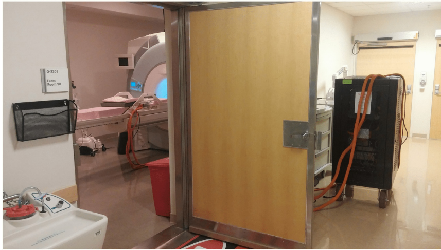
Fig. 2 DOT-MRI system in the clinical MR suite. The optical and electronic components of the DOT-MRI instrument are housed in an instrument rack on pneumatic wheels for easy transport to and from the MR suite. The rack contains all laser sources, the pulsed laser diode driver, all optical switches, the CW detection fiber imaging plate and CCD, PMTs and PMT control-units for TD detection, and TCSPC control instrumentation. When in use, the DOT instrument rack is brought to the control room of the MR suite at the Hospital of the University of Pennsylvania. The fiber bundles then pass into the MRI bore and are incorporated into the clinical breast biopsy RF coil, on which the subject can lie in a prone position to be simultaneously imaged by MRI and DOT.
