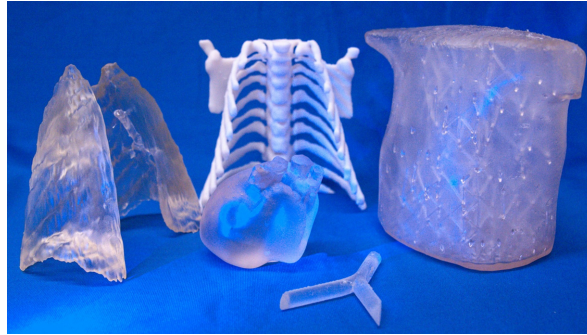
Fig. 3 3D-printed resin structures of the organs in a neonate's thorax to be used for molding, except for the bones (in white)- which were included in the phantom.
