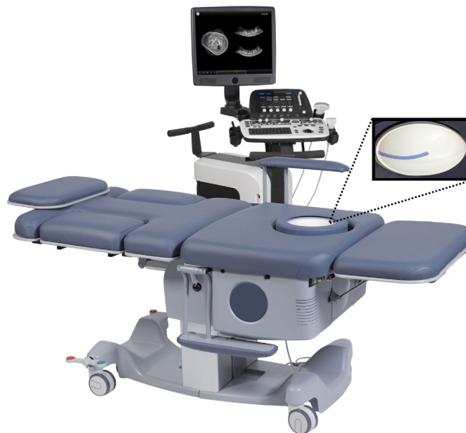
Fig. 1 The SonixEmbrace ABUS system, consisting of the ultrasound PC and scanning platform. Inset shows a top-down view of the transducer dome, with the blue transducer array visible.
