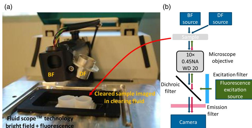
**Fig. 1** Overview of the setup, showing the BF light source and the DF option. (a) DF imaging is achieved by simply relocating the light source into the DF option holder. (b) Schematic representation of the setup and light path.
