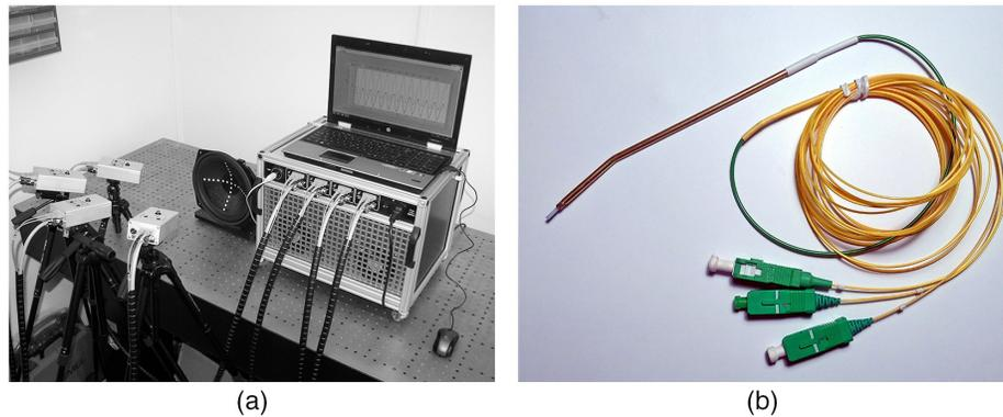
**Fig. 1** (a) The four channel laser-fiber Doppler vibrometer<sup>47</sup> and (b) the handheld probe. The probe, consisting of a ceramic ferrule with the three optical fibers mounted inside a metal shielding sleeve, was connected to one of the four channels of the laser-fiber vibrometer. Two optical fibers are for the forward and return paths of the 1550 nm laser, and one is for the red navigation spot.
