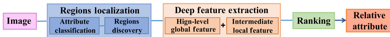
Fig. 1 The pipeline of relative attributes learning, which is composed of regions localization module, deep feature extraction module, and ranking module.
