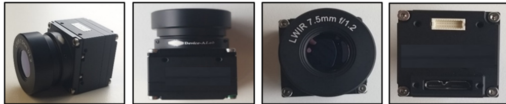
Fig. 8 Prototype thermal VGA camera model for acquiring local facial data.
