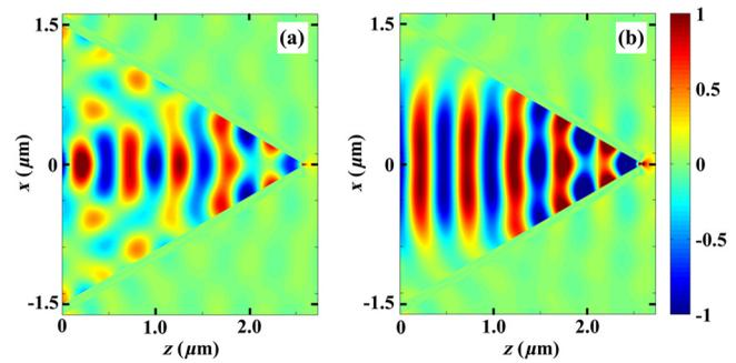
Fig. 2 Distributions of the electric field component  $E_x$  in the TMG (NA = 0.75,  $\lambda = 500 \text{ nm}$ , BW = 9.0 mm): (a) without and (b) with the amplitude modulation.
