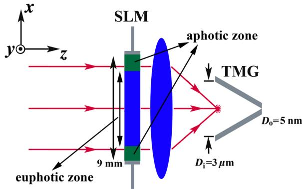
Fig. 1 The schematic diagram of the amplitude modulation method.
