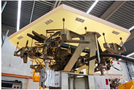
**Fig. 19** Photograph of the European ELT ZERODUR® M1 mirror segment on warping harness. © ESO.
