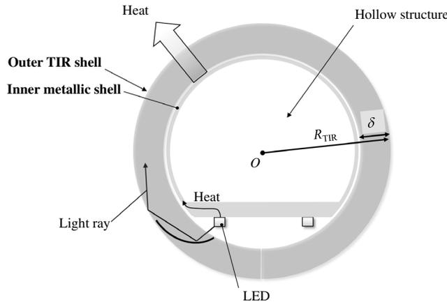
**Fig. 1** Schematic cross-sectional view of concentric shells composed of outer TIR shell and inner metallic shell. The outer TIR shell is assumed to have a uniform thickness of  $\delta$  with an outermost radius of  $R_{TIR}$ . The inner metallic shell with an outermost radius of  $R_{TIR} - \delta$  is assumed to have sufficient thermal conductivity, which makes its temperature distribution uniform.
