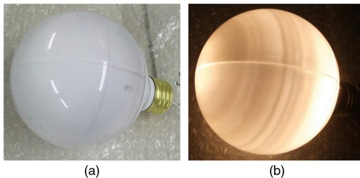
**Fig. 6** Fabricated prototype of large globe LED bulb composed of the concentric shells with outermost diameter of 95 mm. (a) The LED bulb turned off and (b) turned on.
