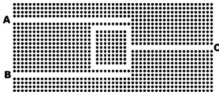
Fig. 20 Construction of 55 \times 23 OR gate with A and B as input. 44
