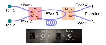
Fig. 3 Schematic of the demonstrator operation. This shows how the illuminated fibers are routed out of the BS and PBS, and the way in which they will light up depending on the switches. The lower image is of the switches on the front panel.
