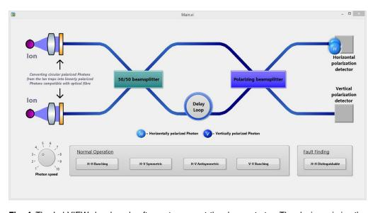
**Fig. 4** The LabVIEW developed software to support the demonstrator. The design mimics the experimental setup, with two ion traps emitting photons that enter the fiber optic circuit. The buttons at the bottom of the image select different entanglement scenarios, which are then played out by the blue circular "photons" over the diagram (Video 2, 468 KB, MOV [URL: https://doi.org/10.1117/1.OE.61.8.081802.2]).).
