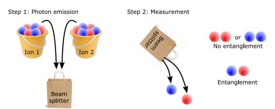
**Fig. 7** Example of a simple scheme for demonstrating entanglement. In step 1, a "photon" from each "ion" is selected blindly and at random, and placed into the "BS." In step 2, the "photons" are measured. If the "photons" match, we know the state of the "ions" and do not achieve entanglement. If they do not match, we cannot tell from which "ion" each "photon" came and entanglement is achieved.
