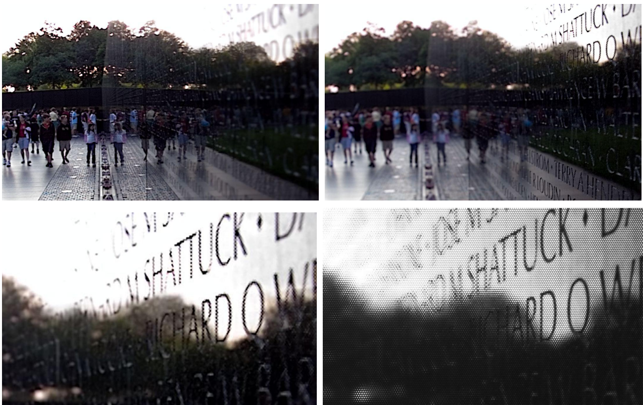
Figure 11. Top row: Two differently focused images based on the same captured Lytro data. Bottom row (left): Zoom in into the text. Notice microlens artifacts in the area of suboptimal focusing. Bottom row (right): Zoom in on the raw image showing that corresponding microimages are actually blurry -- as it should be expected of a plenoptic 1.0 camera.
