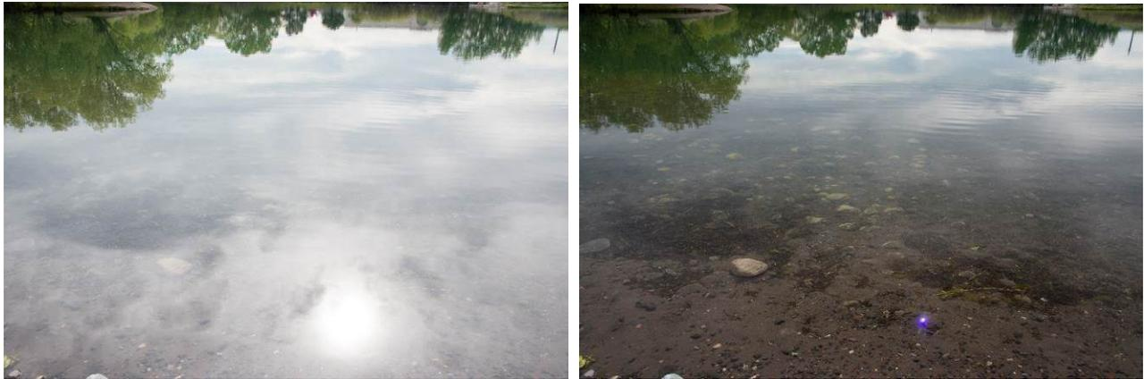
Fig. 5. Reflection from a calm lake surface with the sun  $1.2^\circ$  from the Brewster angle at 1529 UTC, 19 May 2016, solar elevation angle =  $35.8^\circ$ : (left) polarizer rotated for maximum glint brightness; (right) polarizer rotated for minimum glint brightness.
