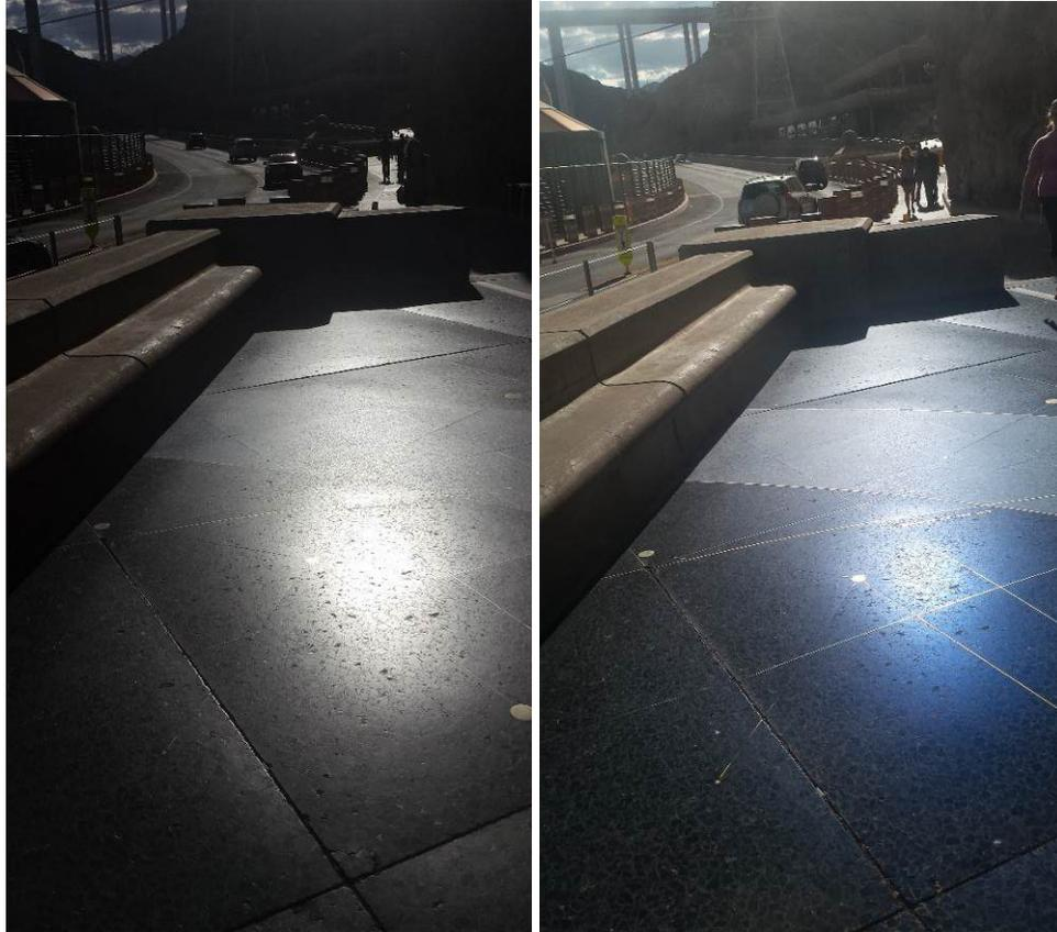
Fig. 10. Smartphone photographs of sun glint on a marble floor near the Hoover Dam monument: (left) no polarizer; (right) looking through Balzer sunglasses oriented to minimize glint brightness.
