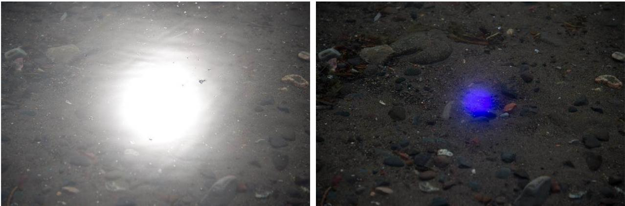
Fig. 6. Zoomed-in images of reflection on a calm lake surface with the sun  $1.2^\circ$  from the Brewster angle at 1529 UTC, 19 May 2016, solar elevation angle =  $35.8^\circ$ : (left) polarizer rotated for maximum glint brightness; (right) polarizer rotated for minimum glint brightness.
