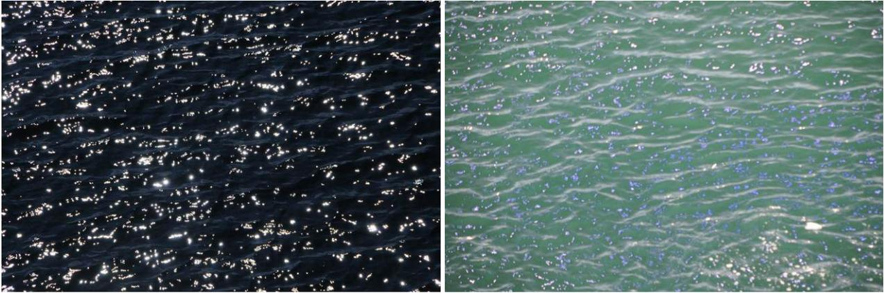
Figure 4. Sun glints observed through a polarizing filter: (left) polarizer oriented approximately horizontal for maximum glint brightness; (right) polarizer oriented approximately vertical for minimum glint brightness.
