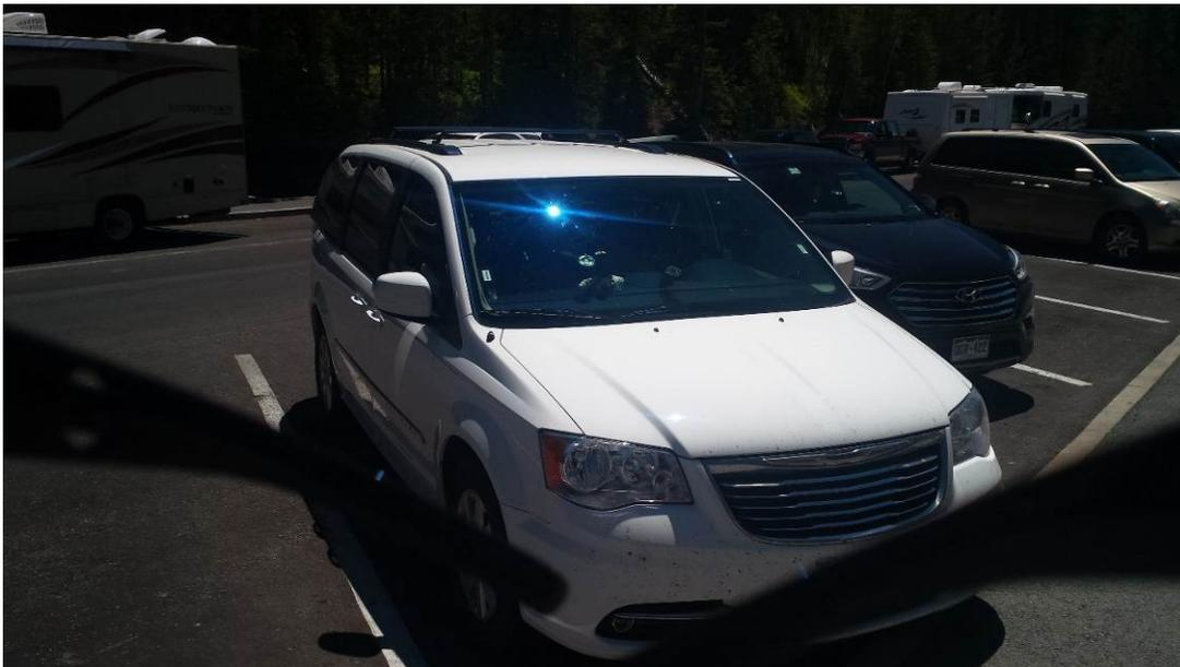
Fig. 11. Smartphone photograph of sun glint on a car windshield looking through Balzer sunglasses oriented to minimize glint brightness.
