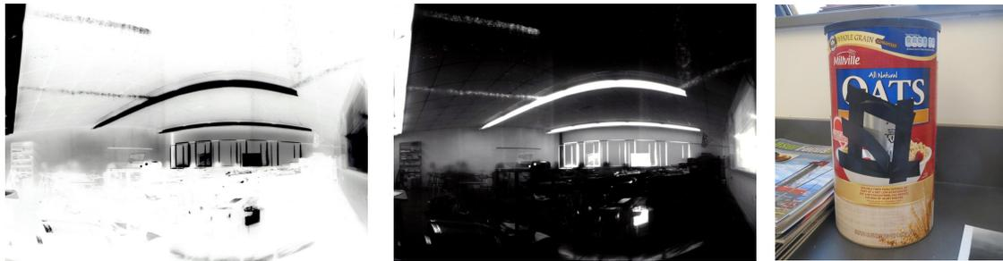
Figure 2 - Roughly 30 minute oatmeal box pinhole camera exposure of classroom (left), inverted version (center) and oatmeal box camera (right).
