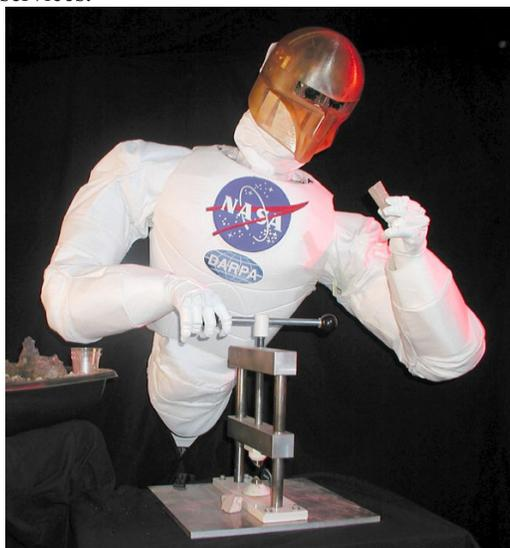
**Figure 8:** The Robonaut I is remotely controlled to perform physical tasks by mirroring the actions of a human (image: NASA Johnson Space Center).
