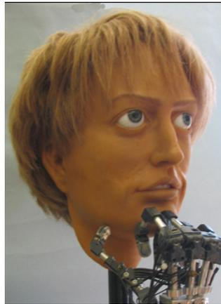
**Figure 4:** A humanlike robot made with Frubber skin making it lifelike. The head (created by David Hanson) and the hand (created by Graham Whitely) shown in this photo are located in the author’s NDEAA lab at JPL.
