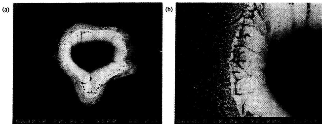
Fig. 5 Pulse laser ablation of stainless steel (X2CrNiMo 17132) at air. Front, 30 fs, 780 nm, 5000 pulses, 1 kHz, linearly polarized,  $16 \text{ Jcm}^{-2}$ . (a) total aspect, (b) detail.
