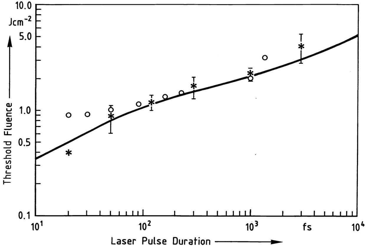
Fig. 3 Threshold fluence  $F_{th}$  vs. laser pulse duration  $\tau$  for the pulse laser ablation of barium aluminum borosilicate glass (Corning<sup>®</sup> 7059, \*) and fused silica (Corning<sup>®</sup> 7940, O) at air. 780 nm, 50 pulses, linearly polarized. The error bars are indicated for barium aluminum borosilicate glass. The solid line corresponds to the simulation for barium aluminum borosilicate glass (Eq. 1) <sup>16</sup>.
