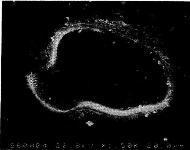
Fig. 2 Pulse laser ablation of barium aluminum borosilicate glass (Corning<sup>®</sup> 7059) at air. 780 nm, 10 pulses, 1 kHz, linearly polarized,  $4\text{ Jcm}^{-2}$ , 20 fs.
