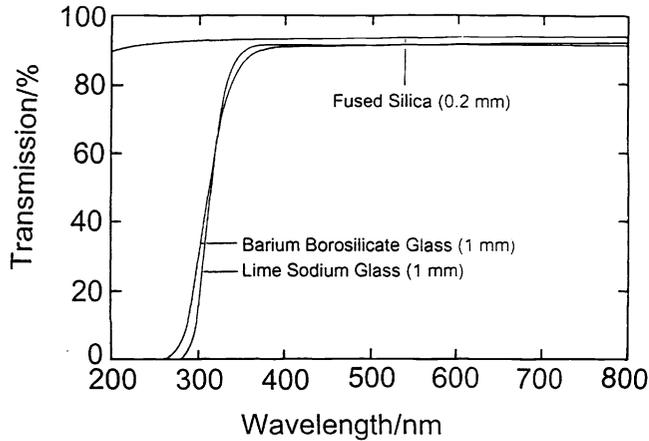
Fig. 1 Ultraviolet and visible transmission of glasses and fused silica.<sup>8</sup>
