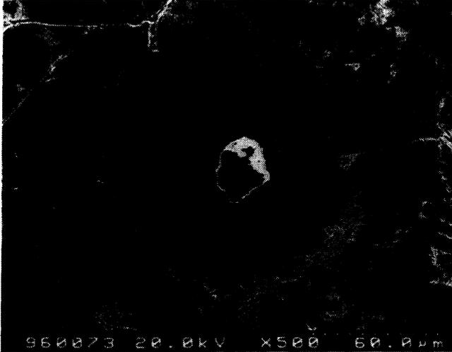
Fig. 6 Pulse laser ablation of stainless steel (X2CrNiMo 17132) at air. Backside, 30 fs, 780 nm, 5000 pulses, 1 kHz, linearly polarized, 16 Jcm<sup>-2</sup>.
