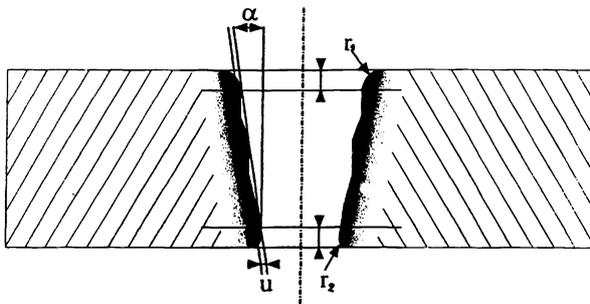
Fig. 7 Precision parameters for laser machining
