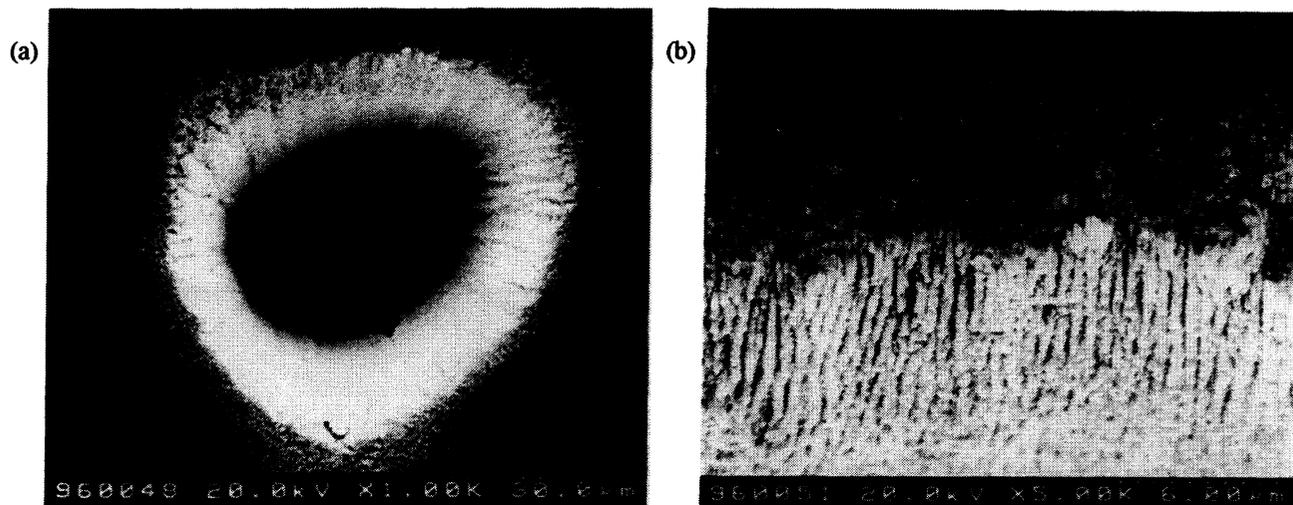
Fig. 4 Pulse laser ablation of stainless steel (X2CrNiMo 17132) at air. Front, 30 fs, 780 nm, 60000 pulses, 1 kHz, linearly polarized,  $3.2 \text{ Jcm}^{-2}$ . (a) total aspect, (b) detail.
