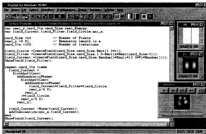
Figure 3. The text window shows a program performing a Fox-Li algorithm 12 which simulates an optical resonator with an internal optical element to induce higher modes (in this case a TEM 01 mode). The upper window shows the function of the internal optical mode filter. Beneath the output of the resonator after 150 roundtrips can be seen and in the bottom window an animation of the mode development is depicted.
