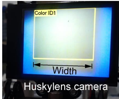
Figure 3. Calibration process by detecting the width of a yellow square.
