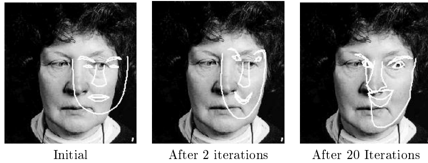
Figure 7. Search using Active Shape Model of a face, given a poor starting point. The ASM is a local method, and may fail to locate an acceptable result if initialised too far from the target
