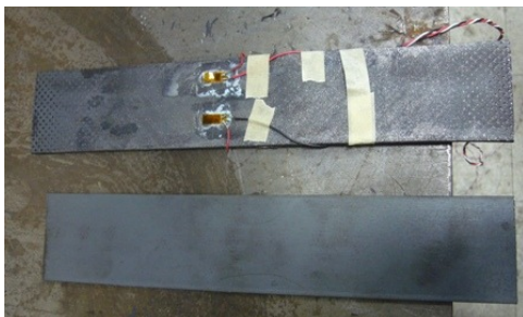
Figure 11. Location of strain gauges (up) and original coupon (bottom)
