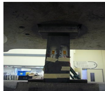
Figure 12. Strain gauges are mounted on the sample strip. Two more gauges are glued to the other side of strip, too.
