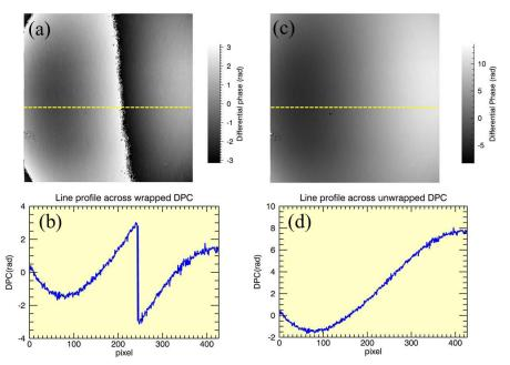
Figure 2. The DPC of the reference image obtained using SHI technique. (a) Wrapped DPC ( $427 \times 427$  pixels), (b) line profile across (a) at y=200<sup>th</sup> pixel. (c) Unwrapped DPC, (d) line profile across (c) at y=200<sup>th</sup> pixel.
