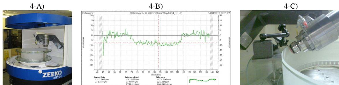
**Fig. 4.** A) Shell mounted on the Zeeko IRP600 machine. B) Example of the influence function of the grolishing process. The circle indicates the grolishing starting point. C) Particular of the Bonnet polishing tool during one of the first grolishing tests to evaluate the suitability of the SSS as interface to the polishing machine.
