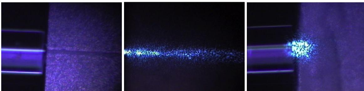
**Figure 2.** (Left) Pump fiber butt to a channel waveguide; (center) green fluorescence propagating in a channel waveguide; (right) fluorescence emitted in a uniform thin film.
