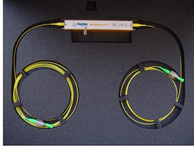
Figure 3. Photline phase shifter of type MPX2000-LN-0.1 with input fiber to the left and output fiber to the right. The phase modulation is realized by setting a voltage to the radiofrequency input at the bottom of the phase shifter housing.
