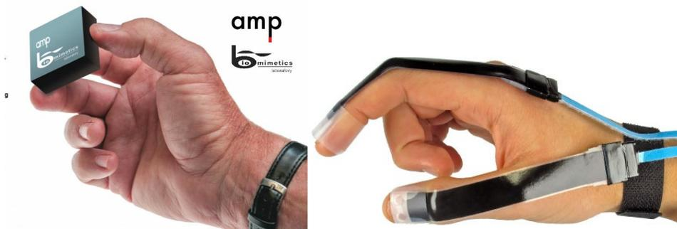
**Figure 13:** Motion capture controller (left) and soft sensor (right)
