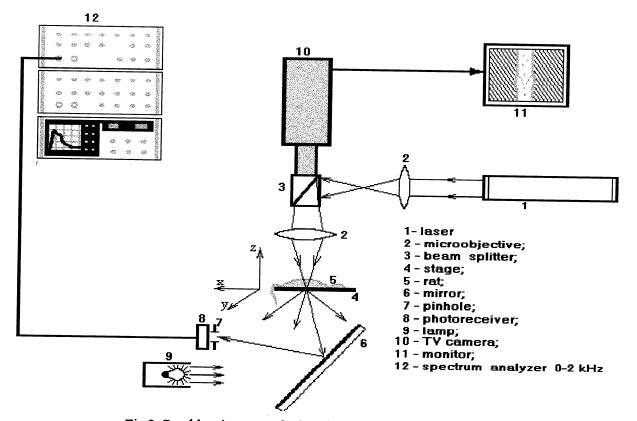
Fig.3. Speckle microscope for lymph flow measurements in micro vessels
