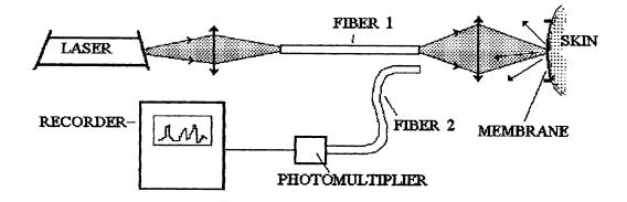
Fig.1. Scheme of speckle-using vibrometer for biovibration monitoring
