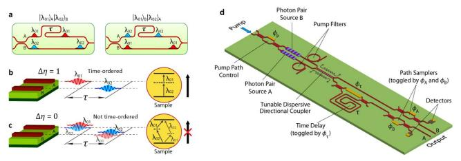
**Figure 3:** (a-c) Dispersion-enabled control over photon time ordering; (d) example of a monolithic photonic quantum circuit where a single dispersive coupler provides multiple functionalities (see text) [4].
