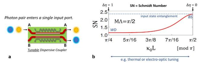
**Figure 2:** Dispersion-enabled control over spectral entanglement; (a) implementation; (b) dependence of output entanglement on coupler response, where  $\Lambda = |\lambda_{02} - \lambda_{01}|$  is the photon pair non-degeneracy and  $\kappa_0$  is the coupling strength at an arbitrary reference wavelength [4].
