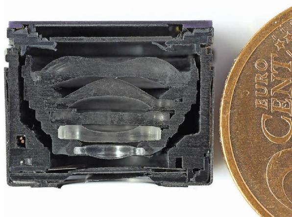
Figure 1. Photograph of a cross section through a camera module for mobile phone; image Carl Zeiss [2]
