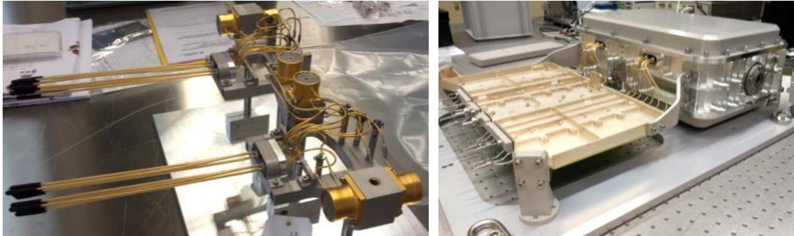
**Fig. 5:** *Left:* LHP-Thermal subsystem ready for integration into the Housing frame. *Right:* Pre assembled pressurized Housing, ready for Thermal Subsystem testing and Integration of Laser optical bench.
