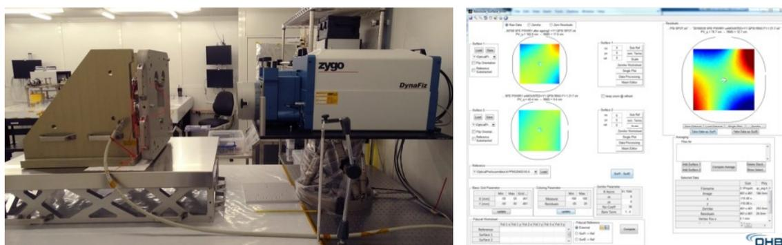
Fig. 12: SFE interferometric measurement setup (left) developed post processing software (right)
