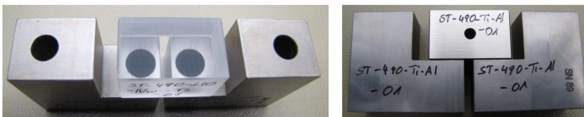
**Fig. 3:** Corresponding prisms with glass-Invar (left) and mirror with titanium-NiP Al alloy (right) samples
