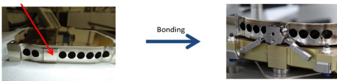
**Fig. 1:** 2 different types of mirror bonding interfaces
