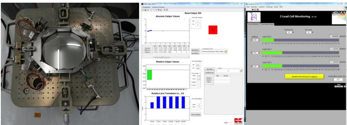
Fig. 8: Example of a prism alignment & bonding MGSE (left) and Alignment Software (right)
