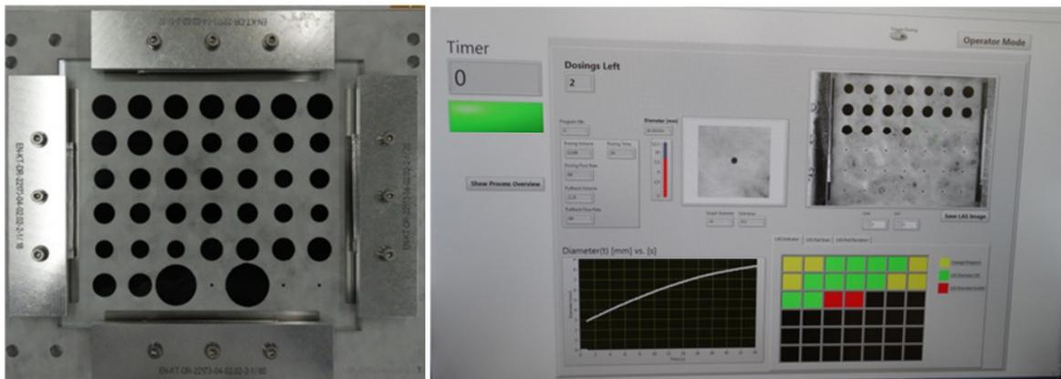
**Fig. 11:** Lot acceptance sample for achievement of gluing pad diameters
