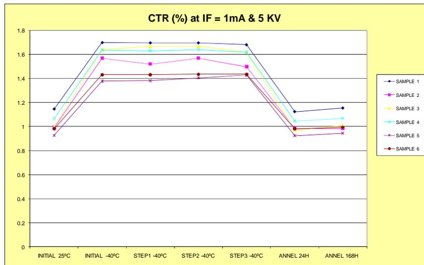
Fig. 4. CTR (at I<sub>F</sub>=1mA and V<sub>RWM</sub>= 5KV) after each gamma radiation step.
